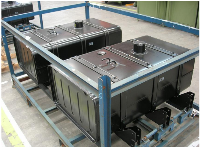
Figure 4: Finished truck's fuel tanks
